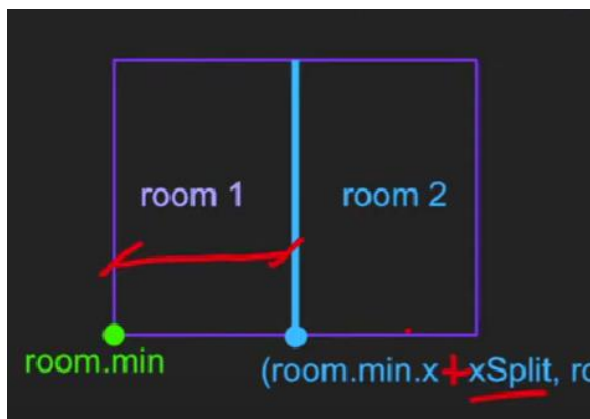
Figure 6: A diagram representing the splitting of a space into two smaller spaces using BSP (Sunny Valley Studio, 2020)
